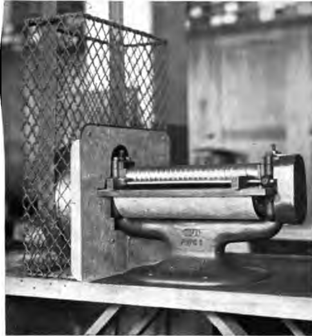
Fig. 1. Strap Cutting Machine with Guarded Knives, Gears and Pulleys.*
